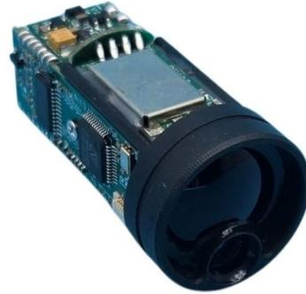
LRF1200A1 laser ranging module is a new lightweight and compact ranging module, operating at a wavelength of 905nm. The maximum range of the product is  $\geq 1200\text{m}$ , using a UART-TTL interface and supporting test software, which is convenient for users to further develop. It has the characteristics of small size, light weight and reliable performance. It can be used in aviation, communications, geology, police, outdoor sports and other occasions.
