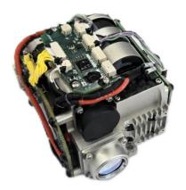
LDR20K1 1064nm Laser Rangefinder & Target Designator. The ranging capability for NATO targets is  $\geq$  3 km. The ranging frequency is  $1\sim20$  Hz. The laser illumination distance is  $\geq2$  km. The pulse width is  $\geq15$  ns  $\pm$  5 ns. The beam divergence angle is  $\leq0.6$  mrad. The weight is  $\leq290$  g.
