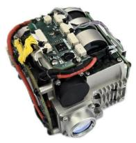
LDR25K1 1064nm Laser Rangefinder & Laser Irradiation. The ranging capability for NATO targets is  $\geq$ 5 km. The ranging frequency is 1~ 20 Hz. The laser illumination distance is  $\geq$  2 km. The pulse width is  $\geq$  15 ns  $\pm$  5 ns. The beam divergence angle is  $\leq$  0.6 mrad. The weight is  $\leq$  380 g.
