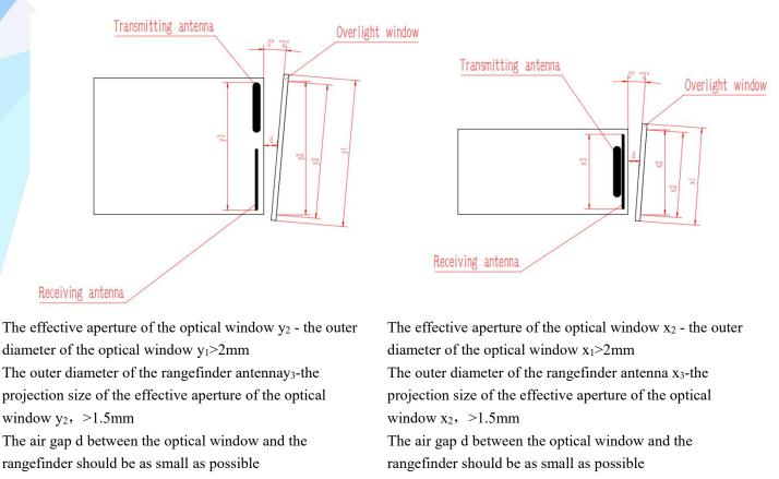
Schematic diagrams of two ways of the external dimensions and placement of the optical window
