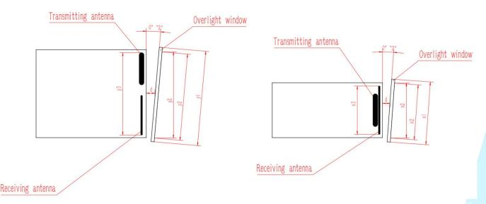
The effective aperture of the optical window  $y_2$  - the outer diameter of the optical window  $y_1 > 2mm$ The outer diameter of the rangefinder antennay<sub>3</sub>-the projection size of the effective aperture of the optical window  $y_2$ , >1.5mm The air gap d between the optical window and the
