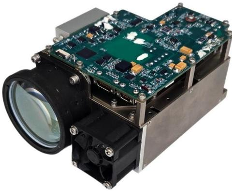
LDR80K2 1064nm Laser Rangefinder & Laser Irradiation. The ranging capability for NATO targets is  $\geq 20$  km. The ranging frequency is 1~ 20 Hz. The laser illumination distance is  $\geq 8$  km. The pulse width is  $\geq 15$  ns  $\pm 5$  ns. The beam divergence angle is  $\leq 0.25$  mrad. The weight is  $\leq 850$  g.
