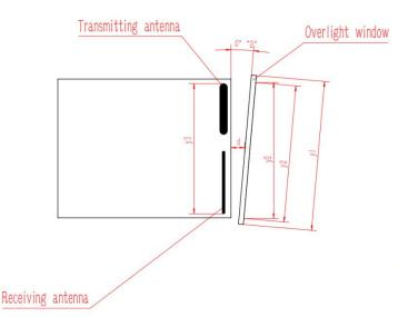
The effective aperture of the optical window  $y_2$  - the outer diameter of the optical window  $y_1$ >2mm
