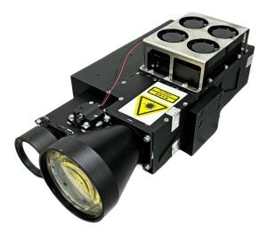
LR160 1064nm 160mJ Laser Target Designator & Laser Ranging System The ranging capability for NATO targets is  $\geq 30$  km. The ranging frequency is 1~ 20Hz. The laser illumination distance is  $\geq 20$  km. The pulse width is  $\geq 15$  ns  $\pm 5$  ns. The beam divergence angle is  $\leq$ 0.2 mrad. The weight is  $\leq 3.3$  kg.
