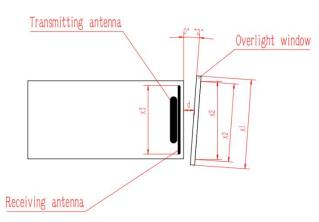
The effective aperture of the optical window  $x_2$  - the outer diameter of the optical window  $x_1 > 2mm$ The outer diameter of the rangefinder antenna  $x_3$ -the projection size of the effective aperture of the optical window  $x_2$ , >1.5mm The air gap d between the optical window and the
